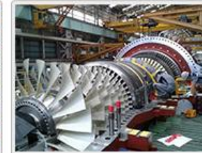
Blade Ring Assembly & Bolt Tightening
