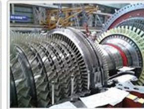
Blade Ring Assembly & Clearance Check
